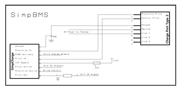
The 5K  $\Omega$  resistor between the SimpCharge Pilot out and SimpBMS is required, do not forget to add this inline.
